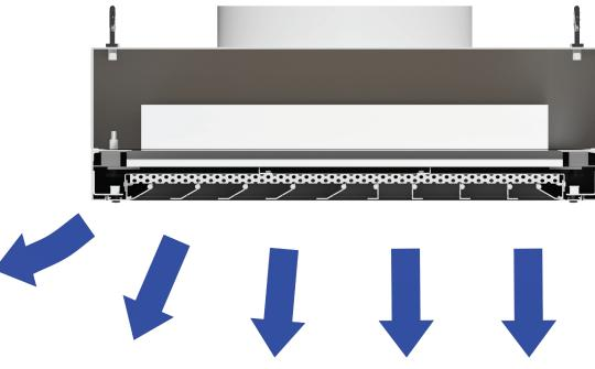
FRFDC with Louvered Face and 1-way half radial airflow pattern (cutaway end view)
